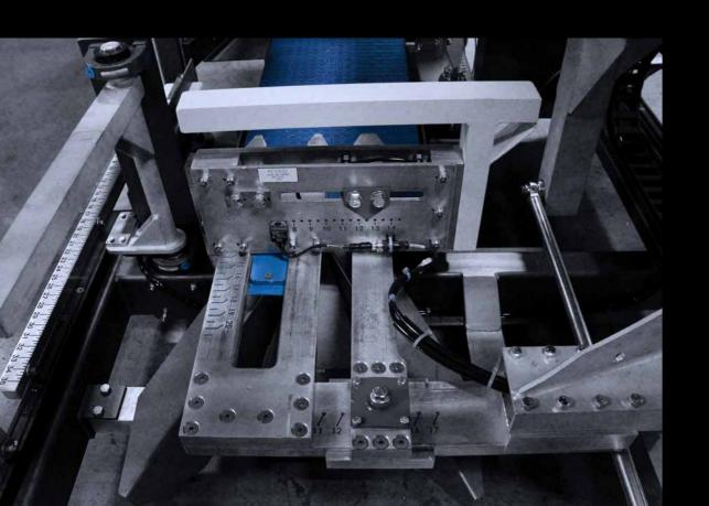
top and side loading of flexible bags with an automatic case packing system with integrated case erector
