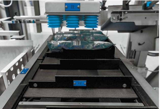
The SPIDER 200 is the ultimate packaging machine for your vertical packaging requirements. It is similar to the SPIDER 100, but used for vertical case loading, rather than a horizontal process.
