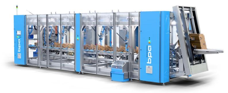
Less material for greater stability. This is the formula used in a wrap around procedure. Using wrap around technology can significantly reduce the costs of packaging material. Wrap around cases or trays are designed to pack products into die cut packaging, which forms directly around the product.
